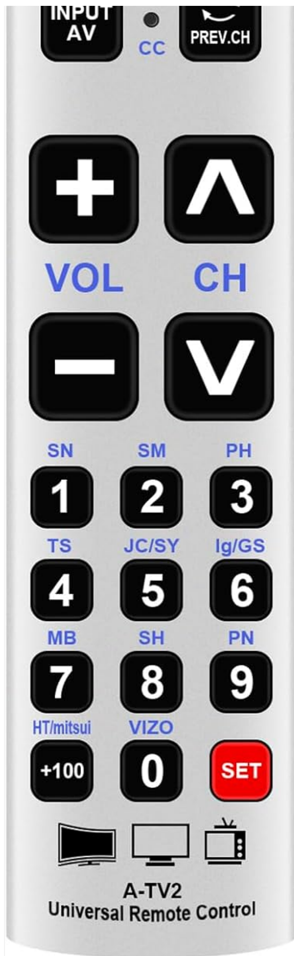
Figure 1: Front view of the ALLIMITY A-TV2 URC-1234ALB Universal Replacement Remote Control. This image displays the full button layout, including the red power button at the top, volume and channel controls in the middle, and the numeric keypad at the bottom, along with input and previous channel buttons.
