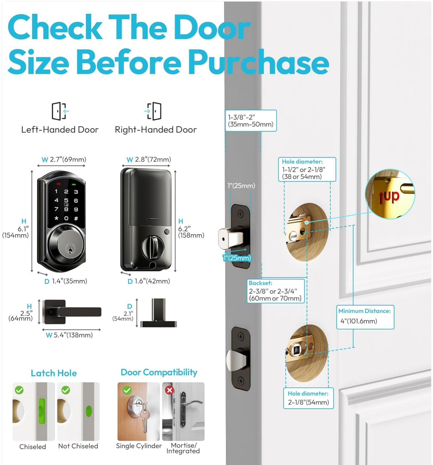
Figure 3: Door measurement and compatibility guide.
