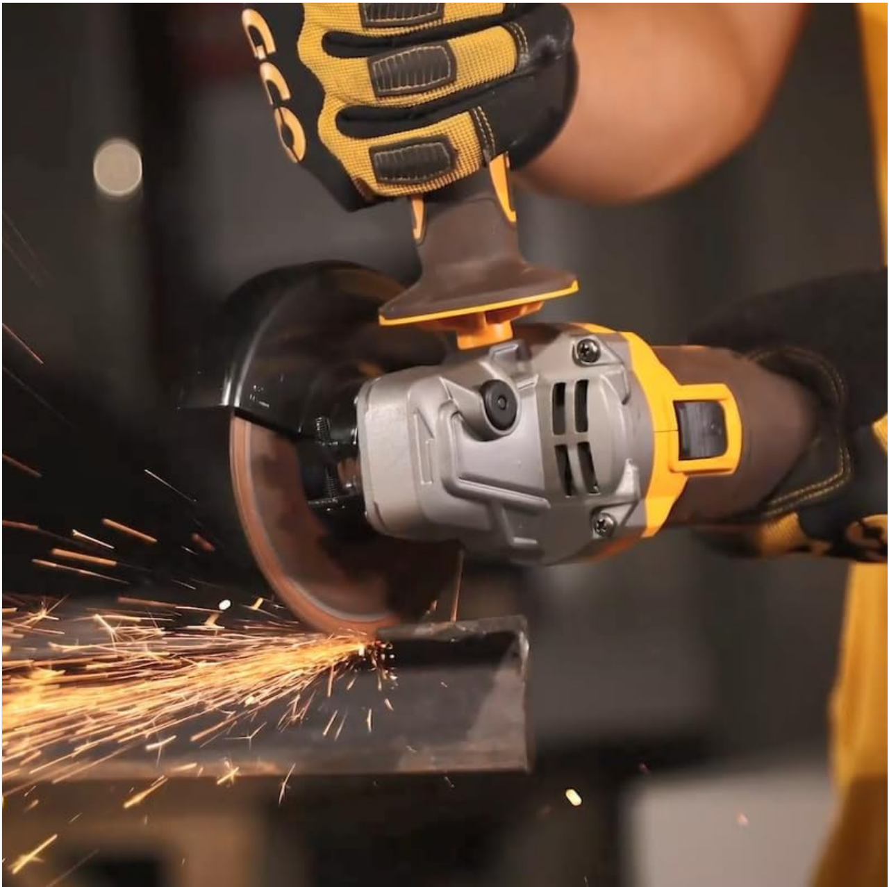
Figure 5: Detailed view of sparks during metal cutting. Always direct sparks away from yourself and others.
