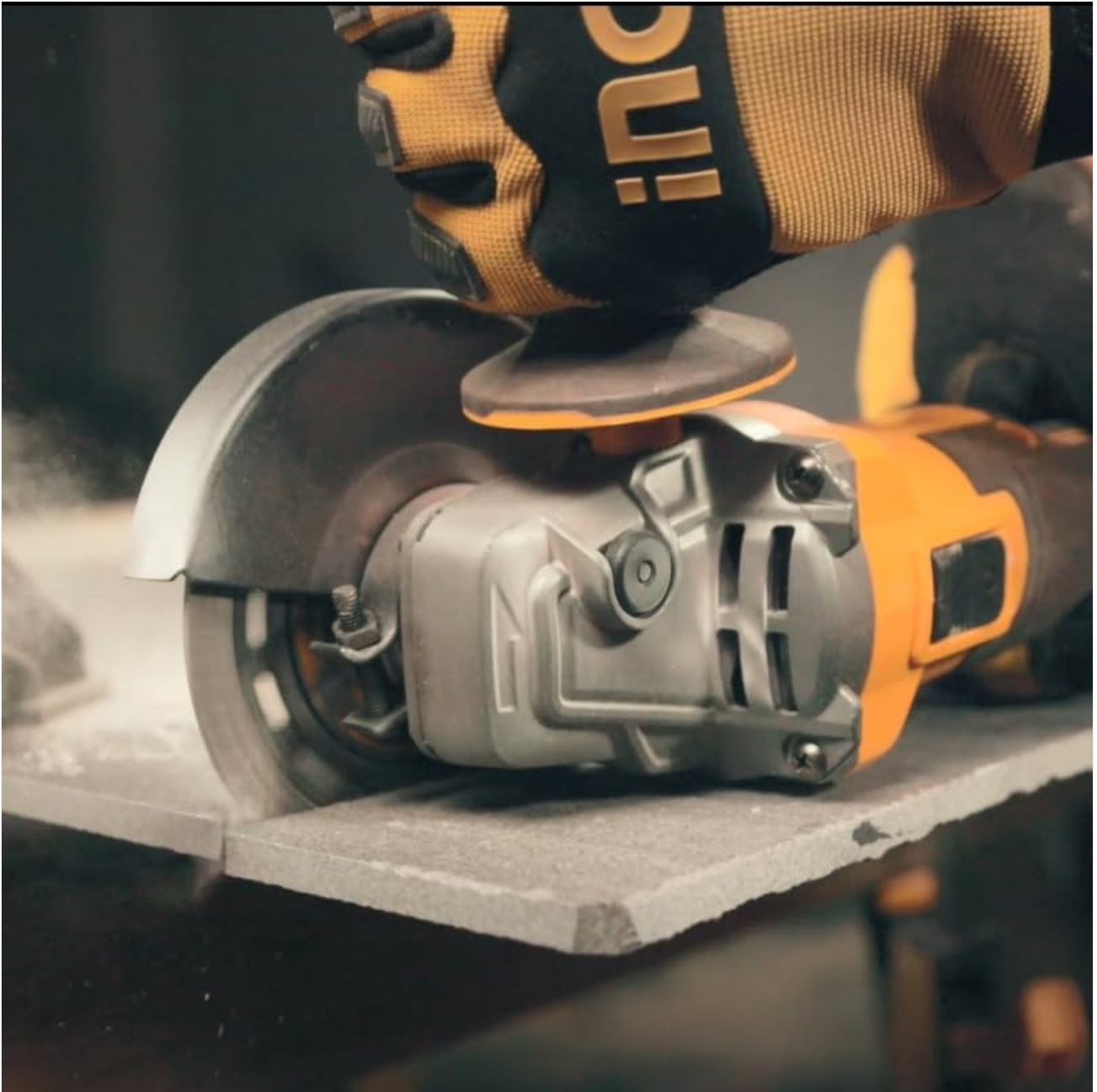
Figure 4: Angle grinder used for cutting tile. Note the dust generated, requiring appropriate respiratory protection.
