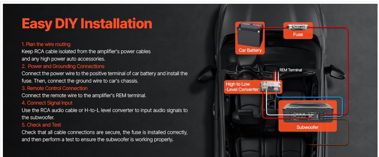
Figure 5: Wiring diagram for typical installation, showing connections to battery, ground, remote, and signal inputs.
