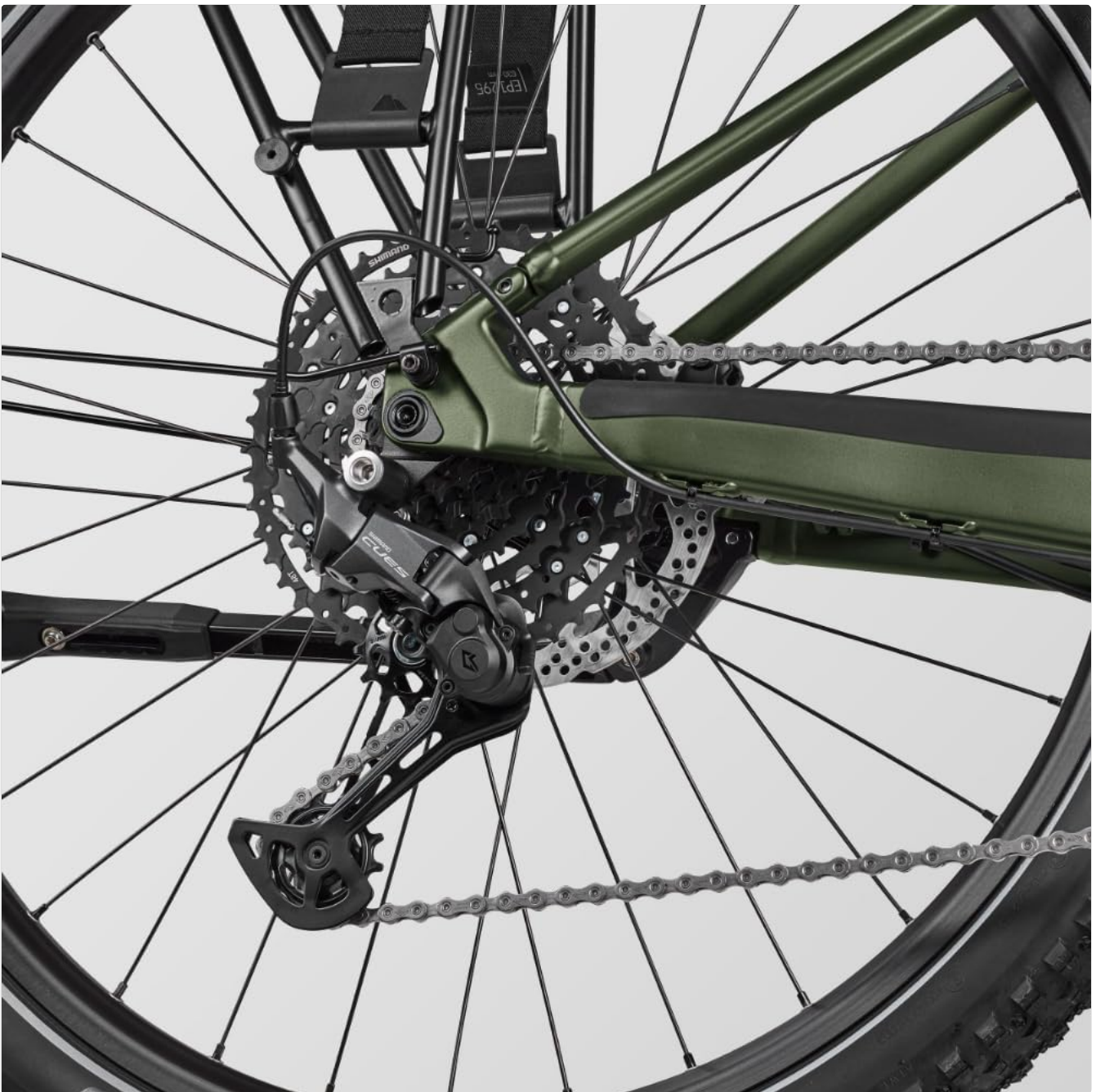
Image 5.1: Detail of the rear derailleur and cassette, components requiring regular cleaning and lubrication.
