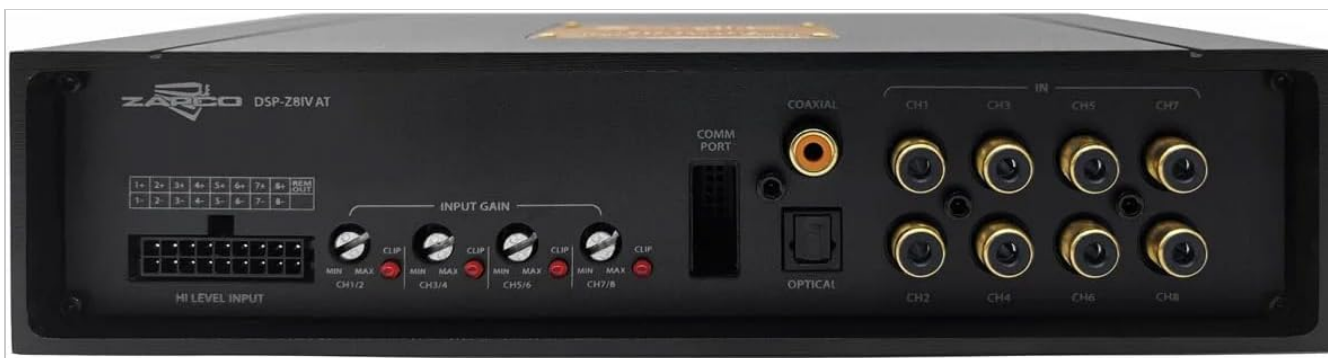
Figure 1: Rear panel view of the Zapco DSP-Z8-IV-AT, illustrating the input section. This includes the High Level Input terminal block, individual Input Gain potentiometers with Clip indicators for channels 1-8, Coaxial and Optical digital input ports, and eight RCA analog input channels (CH1-CH8).
