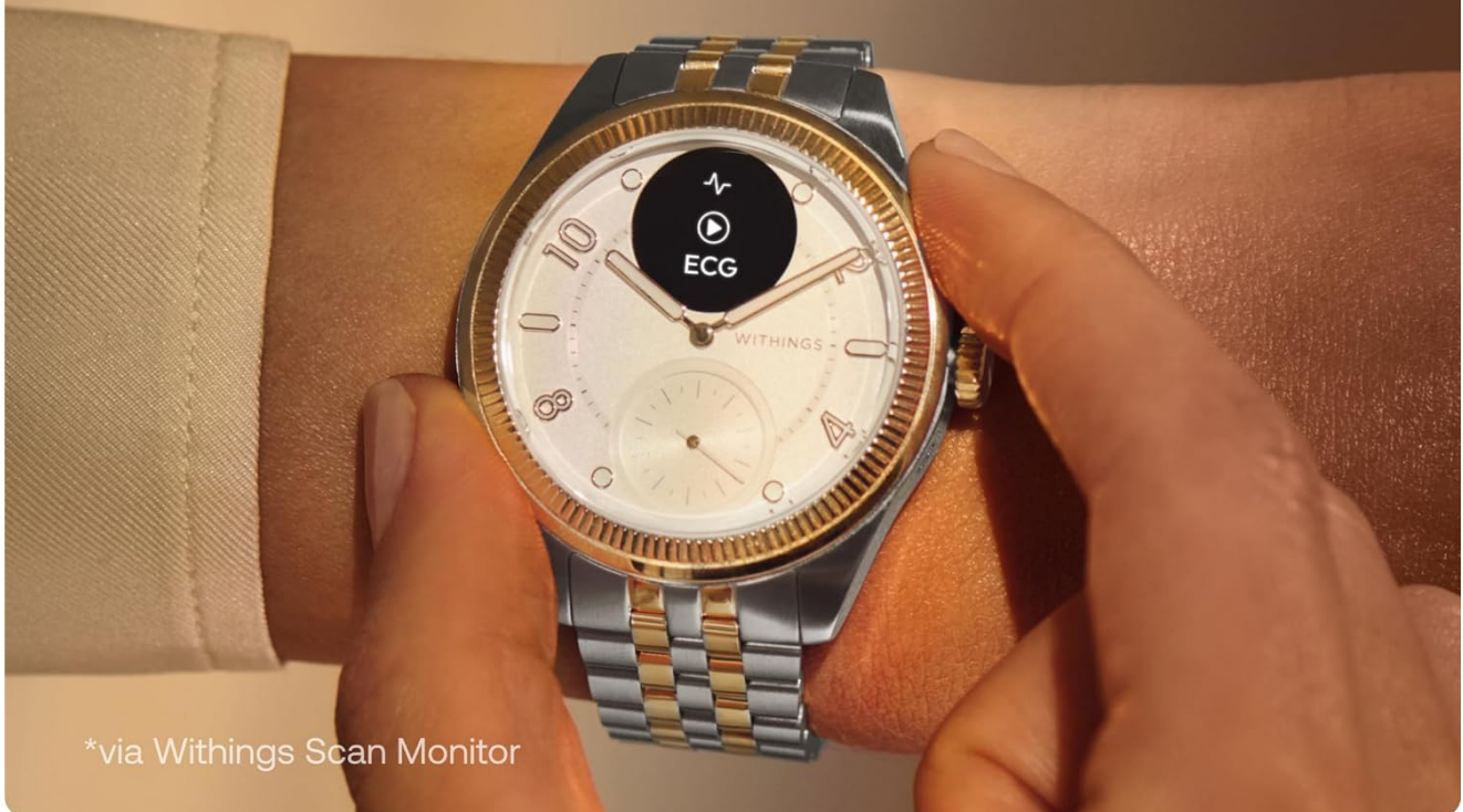
Image 3.1: The Scanwatch Nova Brilliant displaying an ECG reading on its digital screen, indicating the process of heart rhythm analysis.
