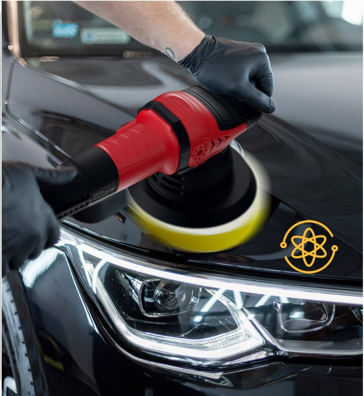
Figure 5: The random orbital motion of the polisher, reducing paint burn risk.
