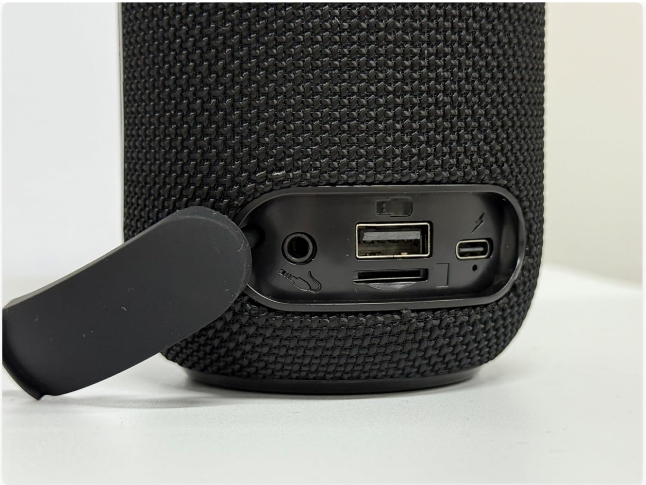
Image 3.1: Detailed view of the speaker's connectivity panel, showing the AUX input, USB port, TF card slot, and Type-C charging port.
