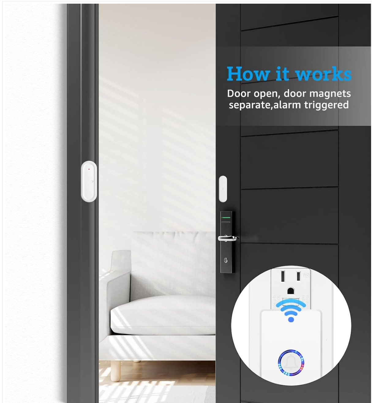
Image 2: Illustration of magnetic sensor installation and operation.
