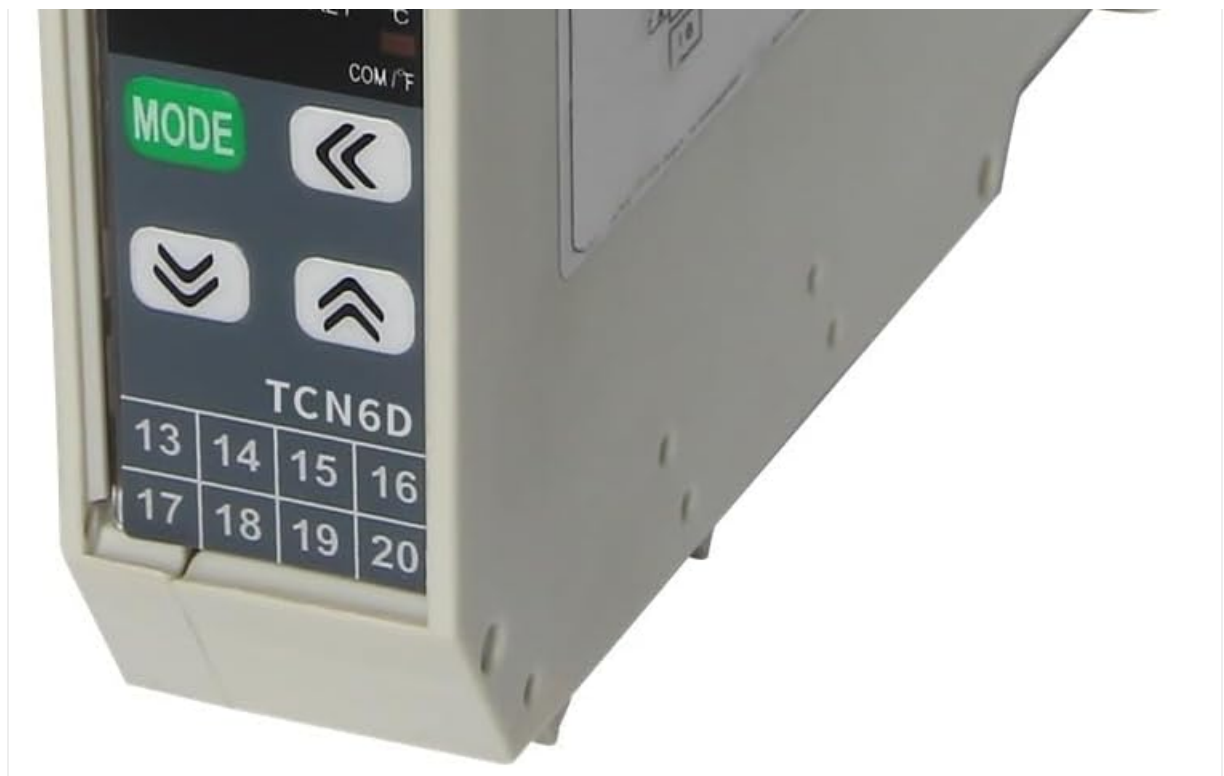
Figure 1: Front View of TCN6-D Controller. This image displays the front panel of the TCN6-D, highlighting the dual digital display for process value (PV) and set value (SV), the 'MODE' button, navigation buttons (up/down/left/right), and the terminal block numbering (1-12 at top, 13-20 at bottom). Status indicators for AT, OUT, AL1, AL2, and C/F are also visible.
