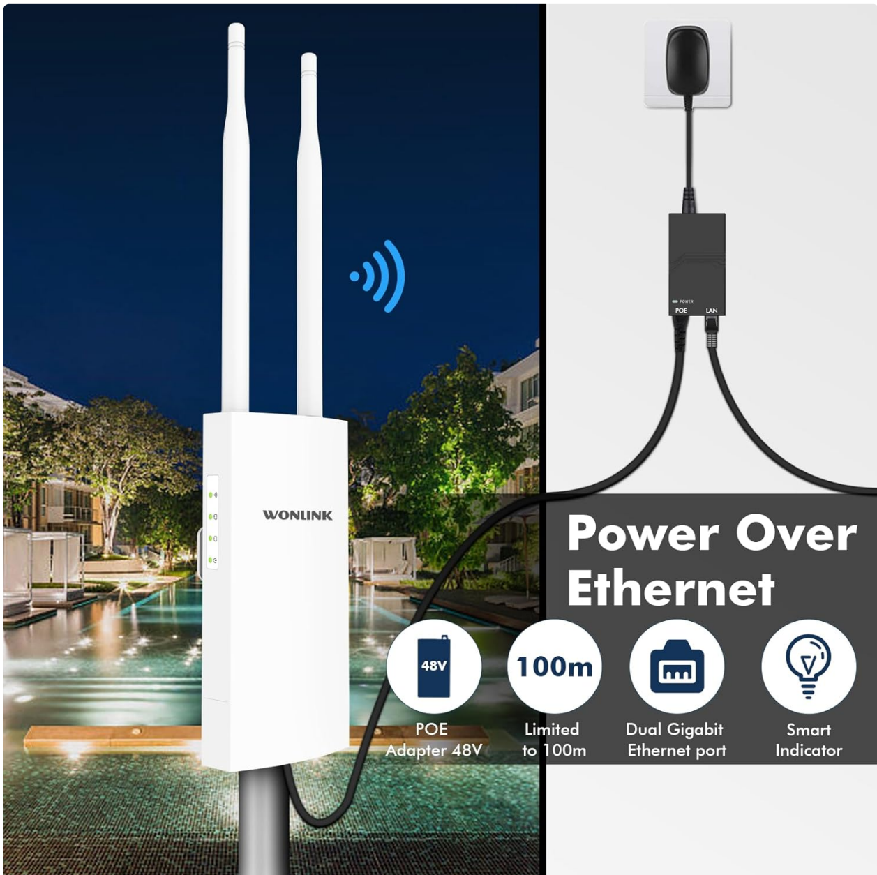
Image 2.1: Diagram illustrating the Power Over Ethernet (PoE) connection setup, showing the extender connected to a PoE adapter and then to a power source and router.
