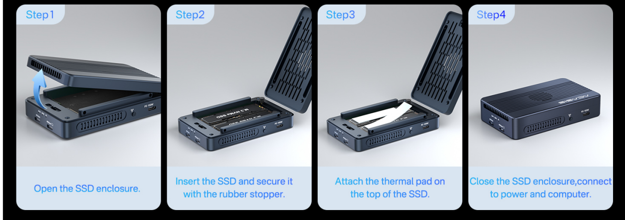
Image: Multiple heat dissipation features of the enclosure.
