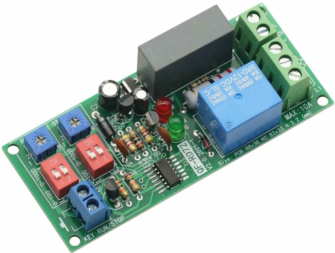
Figure 1: Overview of the Dual Time Adjustable Cycle Delay Timing Relay Module.
