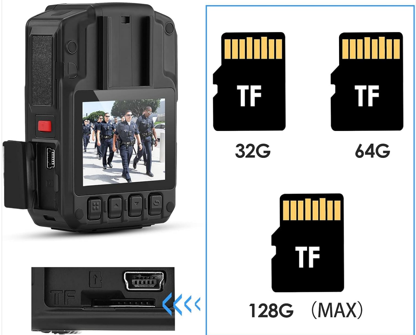
Figure 4.1: External TF Card Storage. This image highlights the TF card slot on the camera and illustrates the compatibility with 32GB, 64GB, and up to 128GB TF cards.
