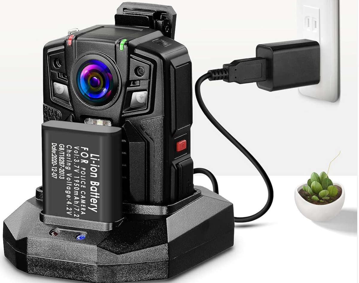
Figure 3.1: High Capacity Battery and Charging Dock. This image illustrates the HD66/D7 body camera connected to its charging dock, with a spare 1950mAh battery also charging. It highlights the dual battery system and charging capabilities.
