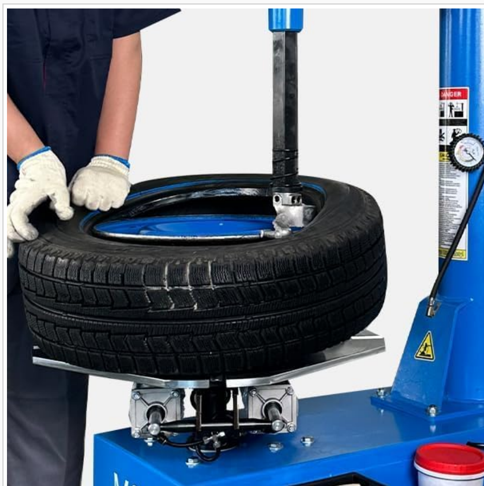
Figure 3: Tire securely clamped on the turntable, ready for demounting or mounting. Note the adjustable clamps.
