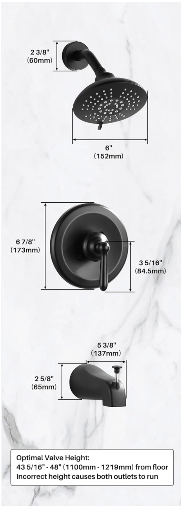
Dimensional drawing of the ARCORA Shower Faucet Set components.
