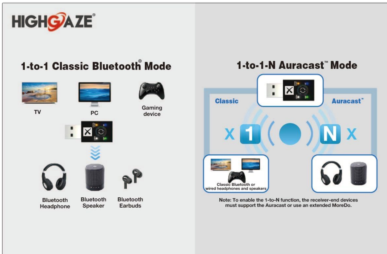
Figure 4: Comparison of 1-to-1 Classic Bluetooth Mode and 1-to-N Auracast Mode.
