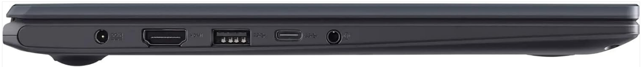
Figure 3: Right side ports including power, HDMI, USB-A, USB-C, and audio jack.
