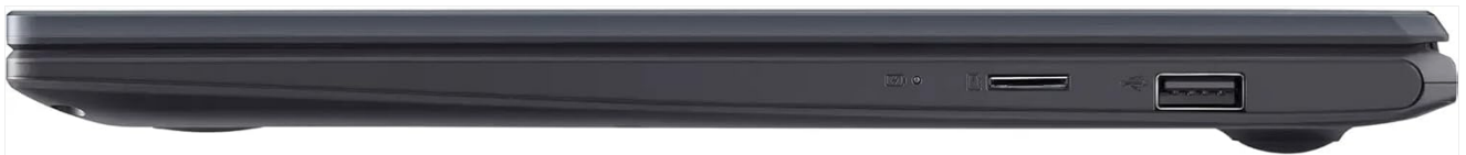
Figure 4: Left side ports including USB-A and Micro SD card slot.
