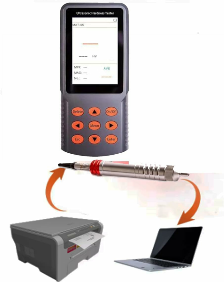
Figure 4.3: Data export functionality. This image illustrates the device's ability to export data, showing it connected to both a printer and a laptop, signifying options for printing or digital transfer of measurement results.
