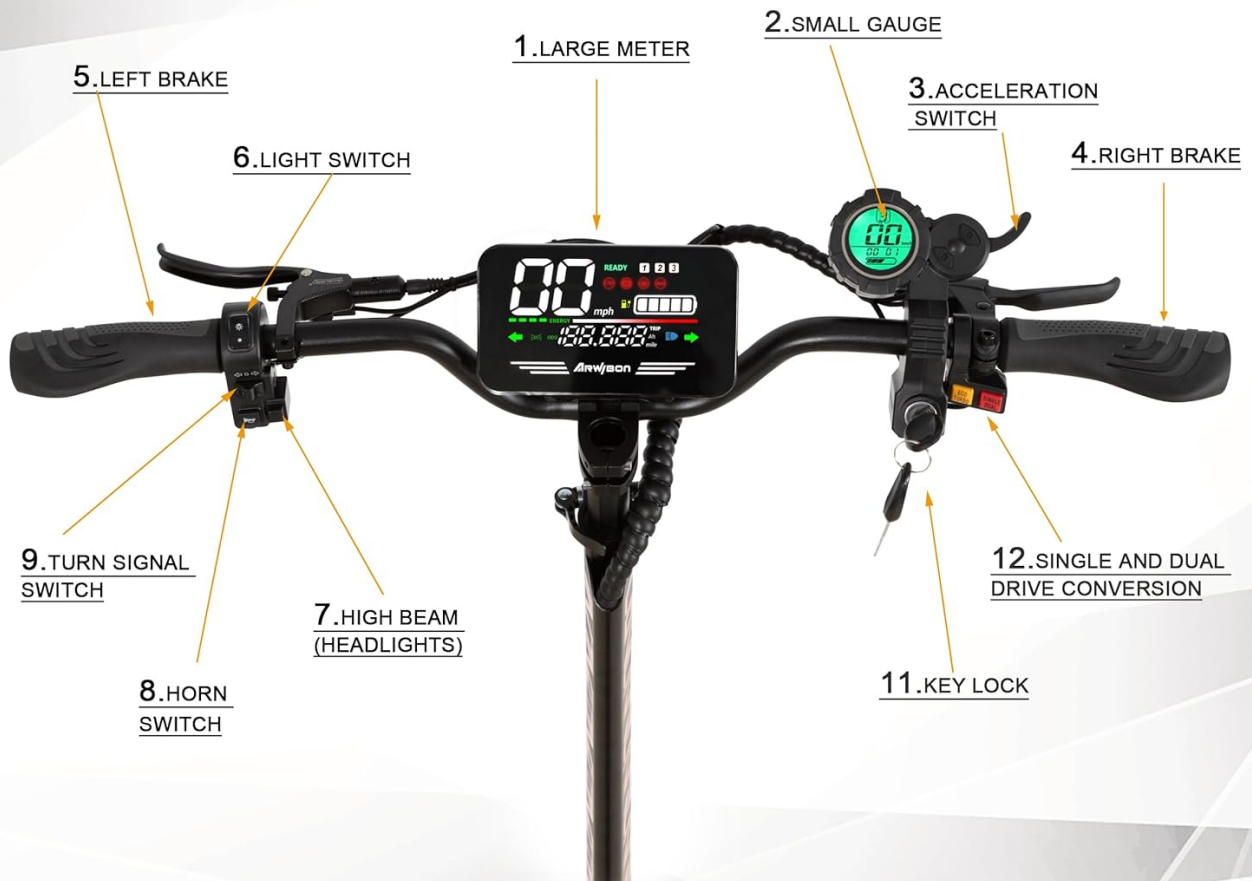
Figure 4.3: Overview of the handlebar controls, including the large meter display, acceleration switch, brake levers, light switch, horn, turn signal switch, high beam, key lock, and single/dual drive conversion switch. Speed modes G1 (16 mph), G2 (38 mph), and G3 (47 mph) are indicated.
