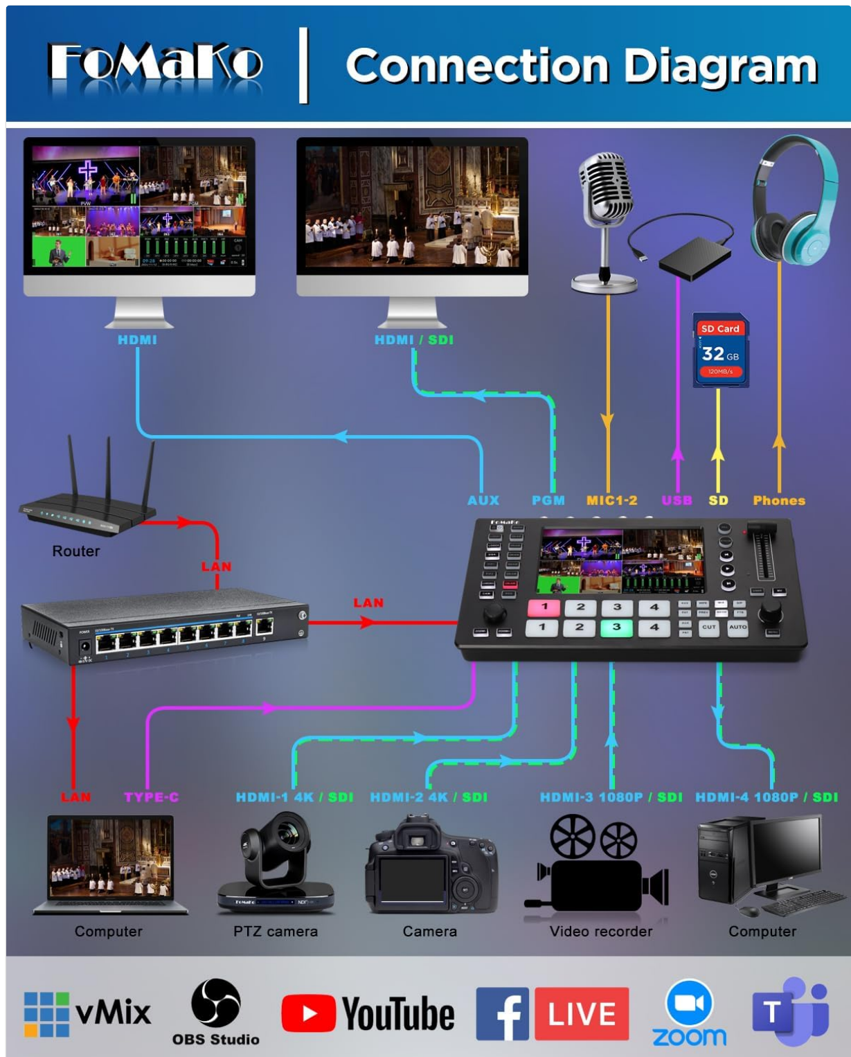
Image 3.2: A visual guide for connecting various devices such as cameras, computers, monitors, and audio equipment to the M4 switcher.
