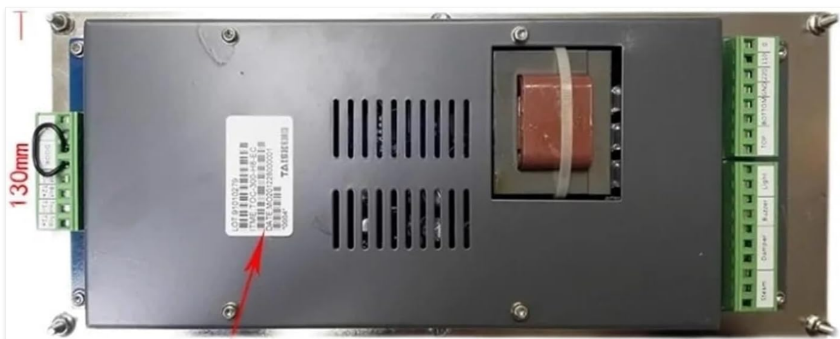
Figure 4.1: Rear view of the TOC-300-H8-EC Motherboard. This image highlights the various connection terminals for power, heating elements (TOP, BOTTOM), light, buzzer, damper, and steam, which are crucial for correct installation.
