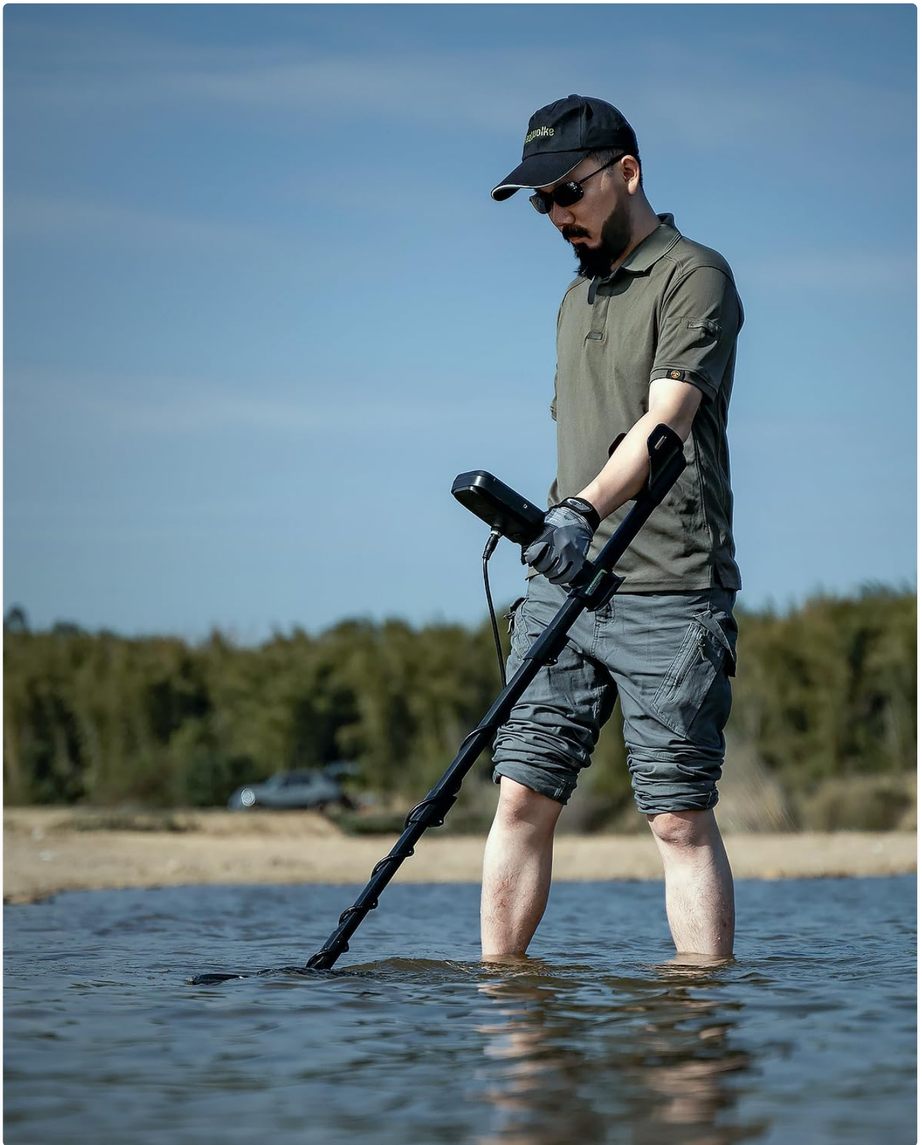
Figure 3.5: The waterproof Double-D coil allows for detection in shallow water.
