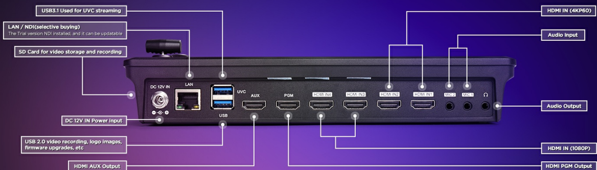
Image: FoMaKo M1 Multi-Interfaces Diagram. This detailed diagram highlights the various input and output interfaces of the M1 switcher, including HDMI, USB, LAN, and audio ports, with labels indicating their functions.
