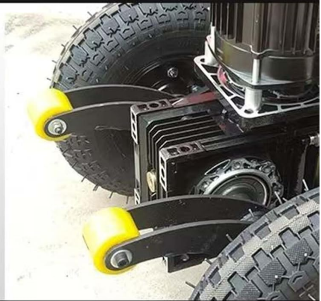
Figure 4: Detail of the robust tire tripod bracket and double-layer S swing arm.
