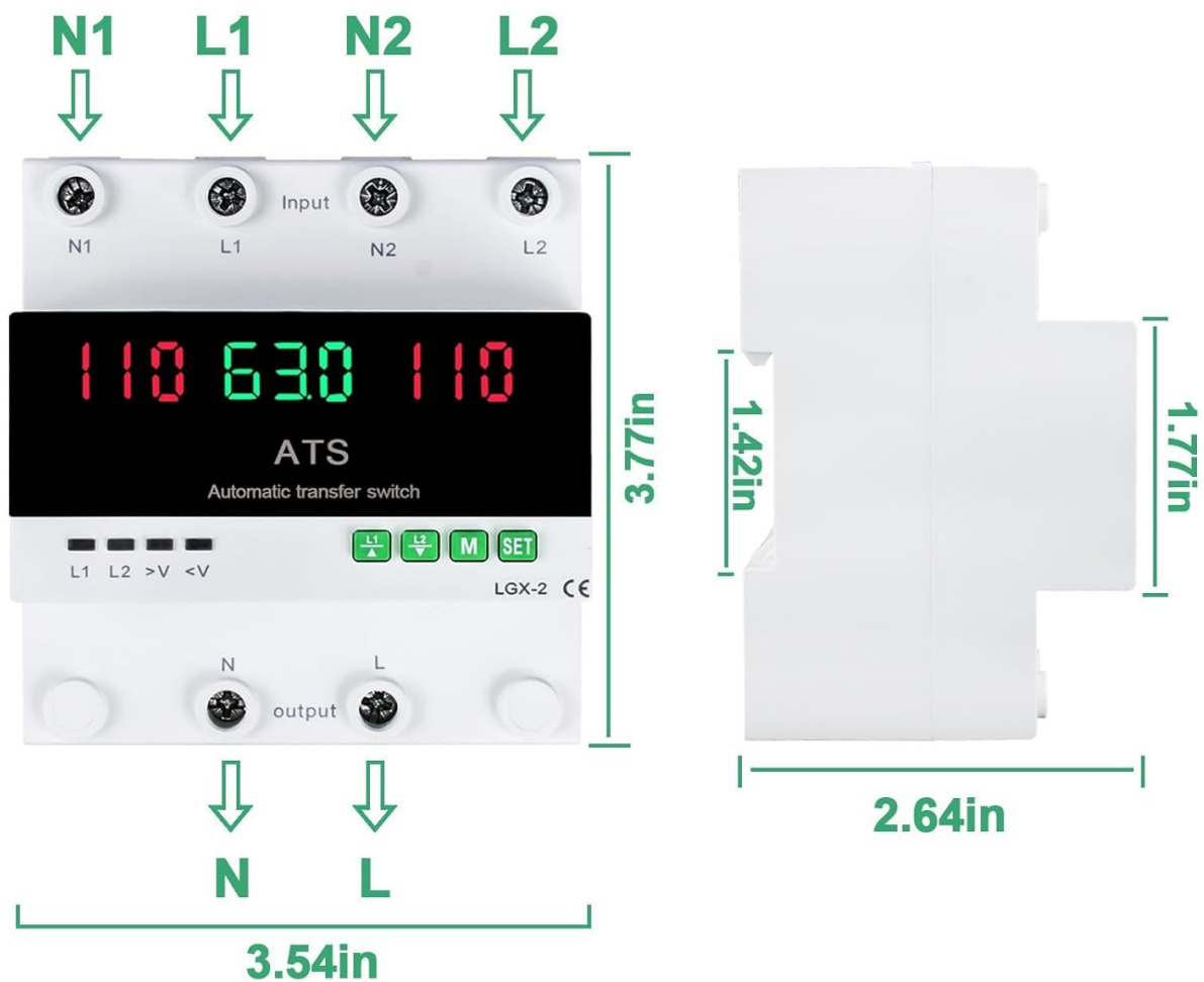
Figure 2: Dimensional Drawing. This diagram illustrates the physical dimensions of the Sekelo SK018 transfer switch, including its height, width, and depth, along with the spacing of input and output terminals.
