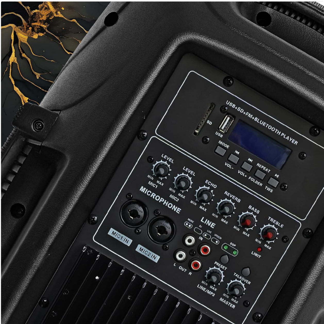
Image 4.1: Detailed view of the active speaker's control panel.
