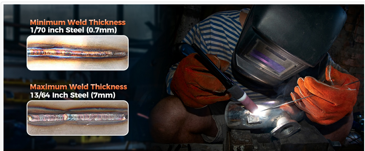
Figure 5.3: Example of TIG welding in progress.
