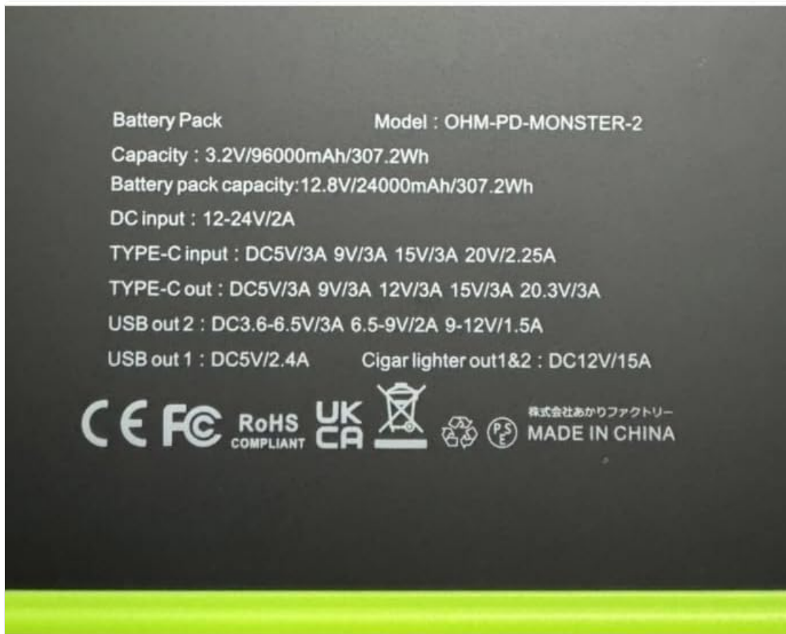
Image: Back label of the OHM-PD-MONSTER-2 displaying detailed electrical specifications and certifications.
