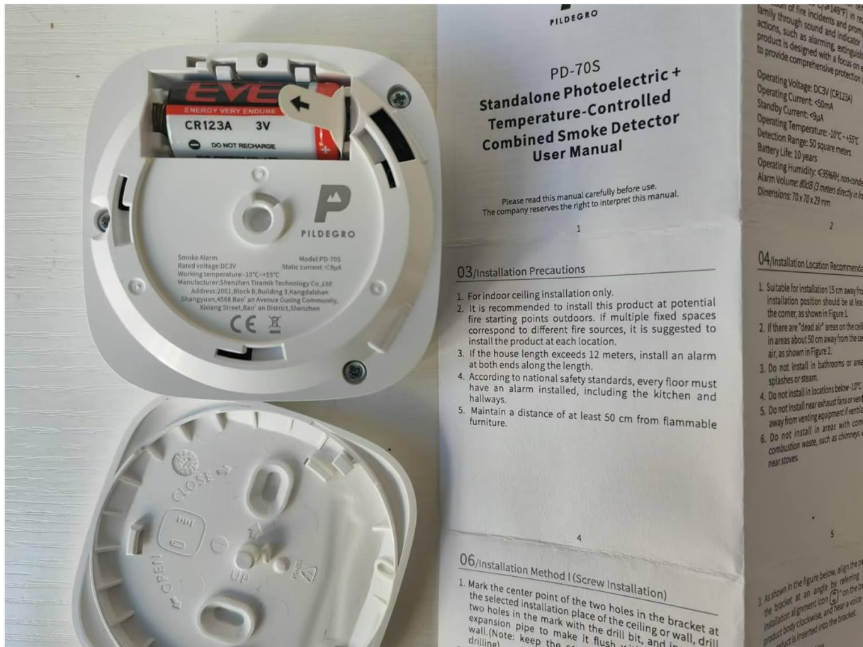
Image: Detailed view of the battery installation and a portion of the manual showing screw installation instructions.
