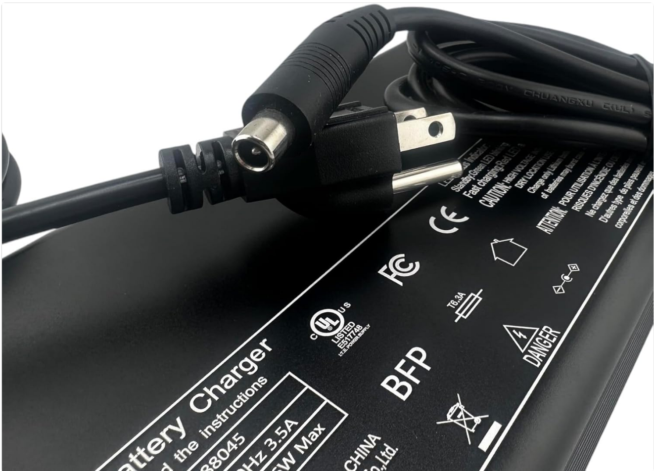
Image 4.1: Close-up of the charger's output connector. This image provides a detailed view of the charging port, which connects to the scooter, and the adjacent AC power input port.
