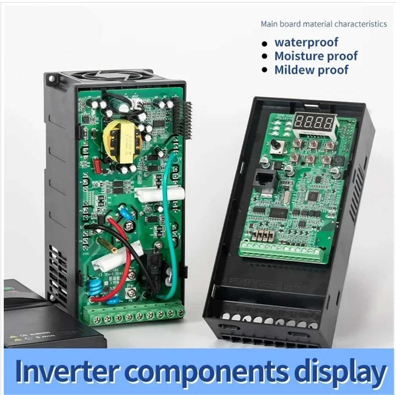
Figure 3.2: Inverter Components Display. This image shows the internal components of the SU600 VFD, emphasizing the main board's characteristics: waterproof, moisture-proof, and mildew-proof design for enhanced durability in various environments.
