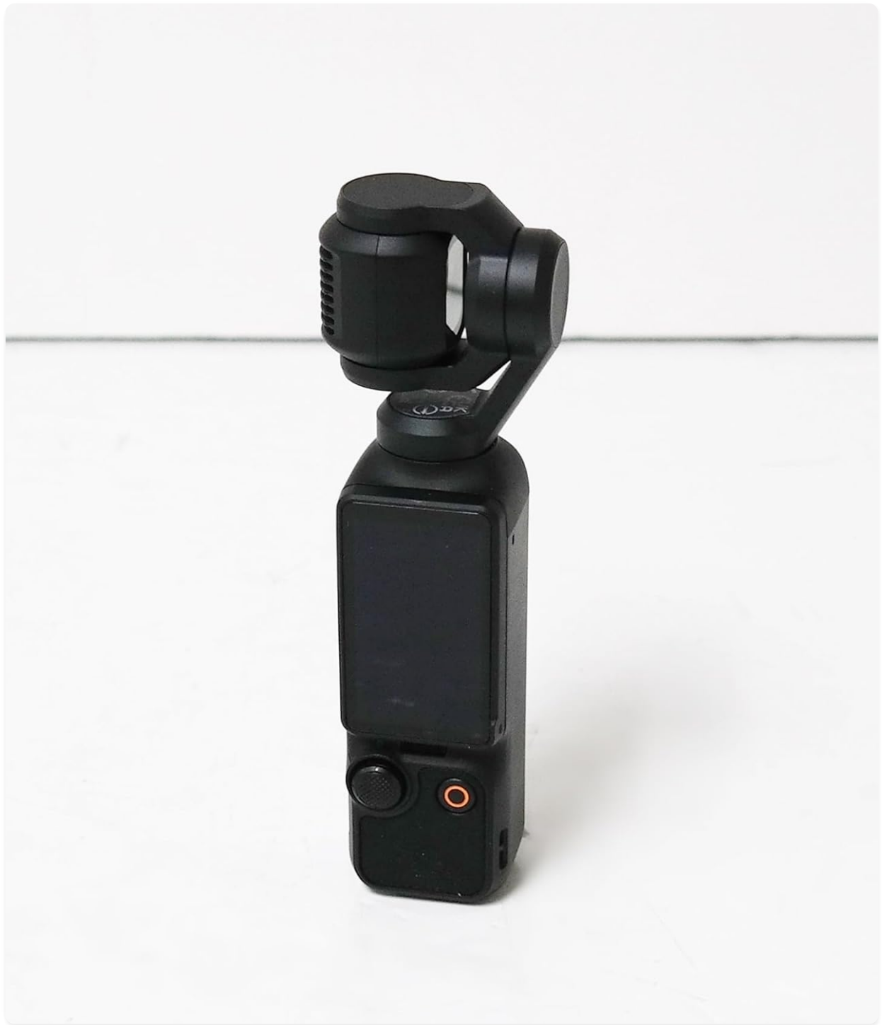
Figure 2: The DJI Osmo Pocket 3 with the wide-angle lens magnetically attached to the camera. The lens expands the field of view for capturing broader scenes.
