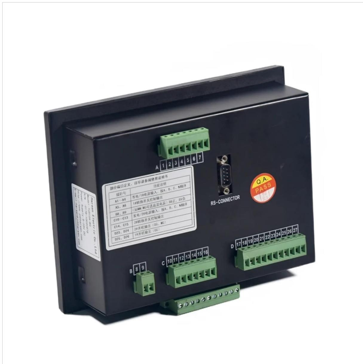
**Image Description:** This image shows the rear of the TU510A control panel, revealing multiple green terminal blocks for electrical connections. These blocks are clearly numbered (e.g., 1-7, 8-9, 10-16, 17-27) for various inputs and outputs. A DB9 'RS-CONNECTOR' is visible on the upper right, indicating serial communication capability. A 'Q.A. PASS' sticker is also present, signifying quality assurance. A label with Chinese text provides connection details.
