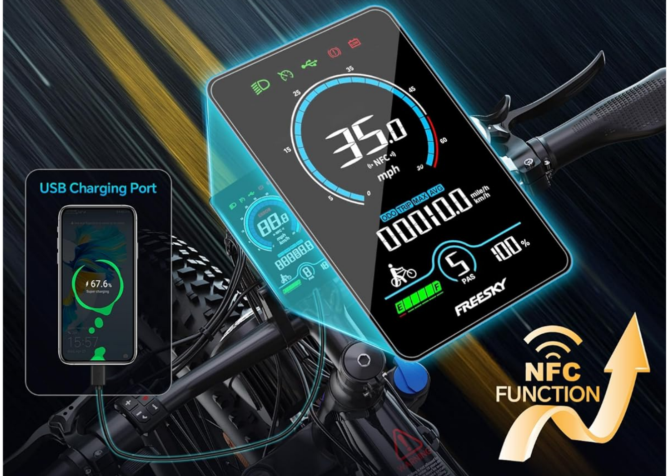
Image: The e-bike's LCD display, showing various metrics and the integrated USB charging port.
