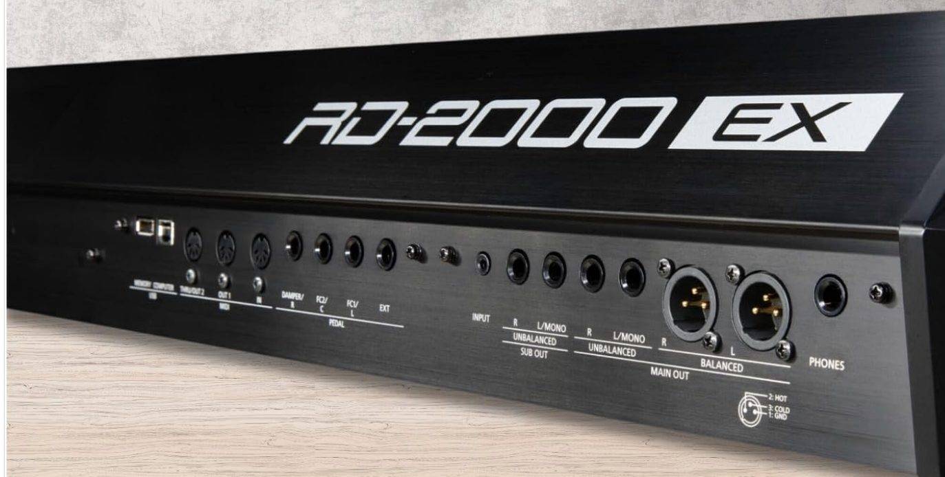
Image: Rear panel of the Roland RD-2000 EX, showing various input/output connections including power, pedal, and audio outputs.
