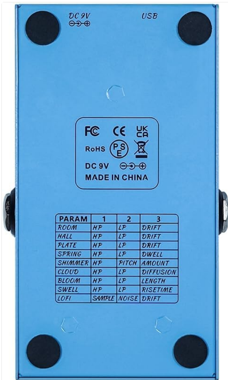
Image: Bottom view of the pedal displaying the parameter function table.
