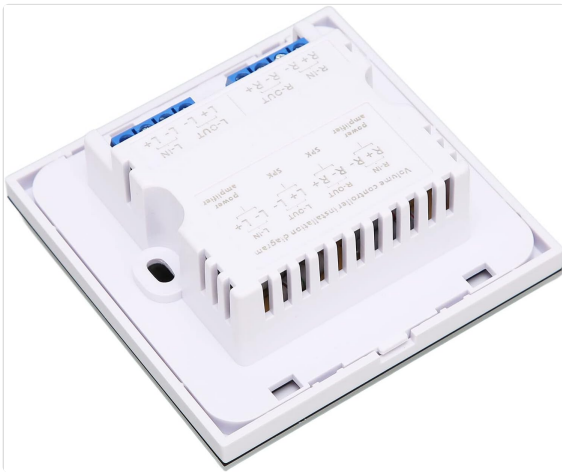
Figure 2.3: Rear view of the Dioche Volume Controller, displaying the input and output wiring terminals (R-IN, R-OUT, L-IN, L-OUT) and a printed installation diagram for connecting to a power amplifier and speakers.
