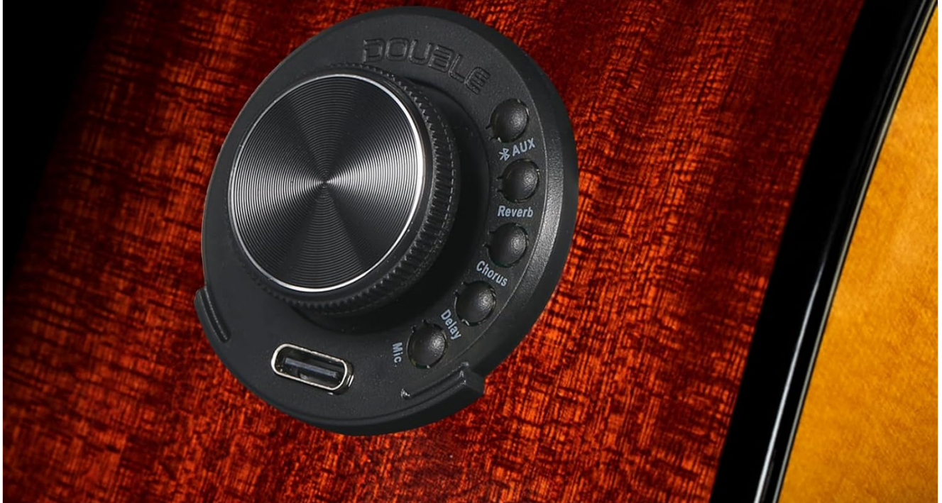
Figure 3.1: The preamp unit installed on a guitar, demonstrating its on-board nature and the necessity for guitar modification.
