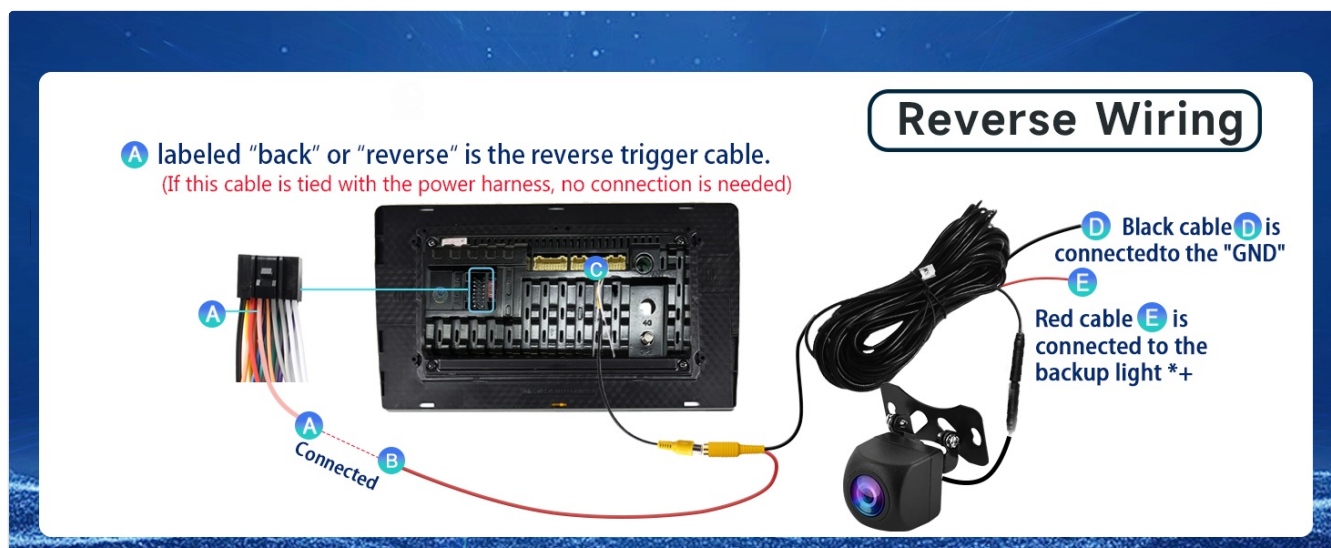
Image 4.1: Detailed wiring diagram for connecting the HD backup camera to the car stereo system.
