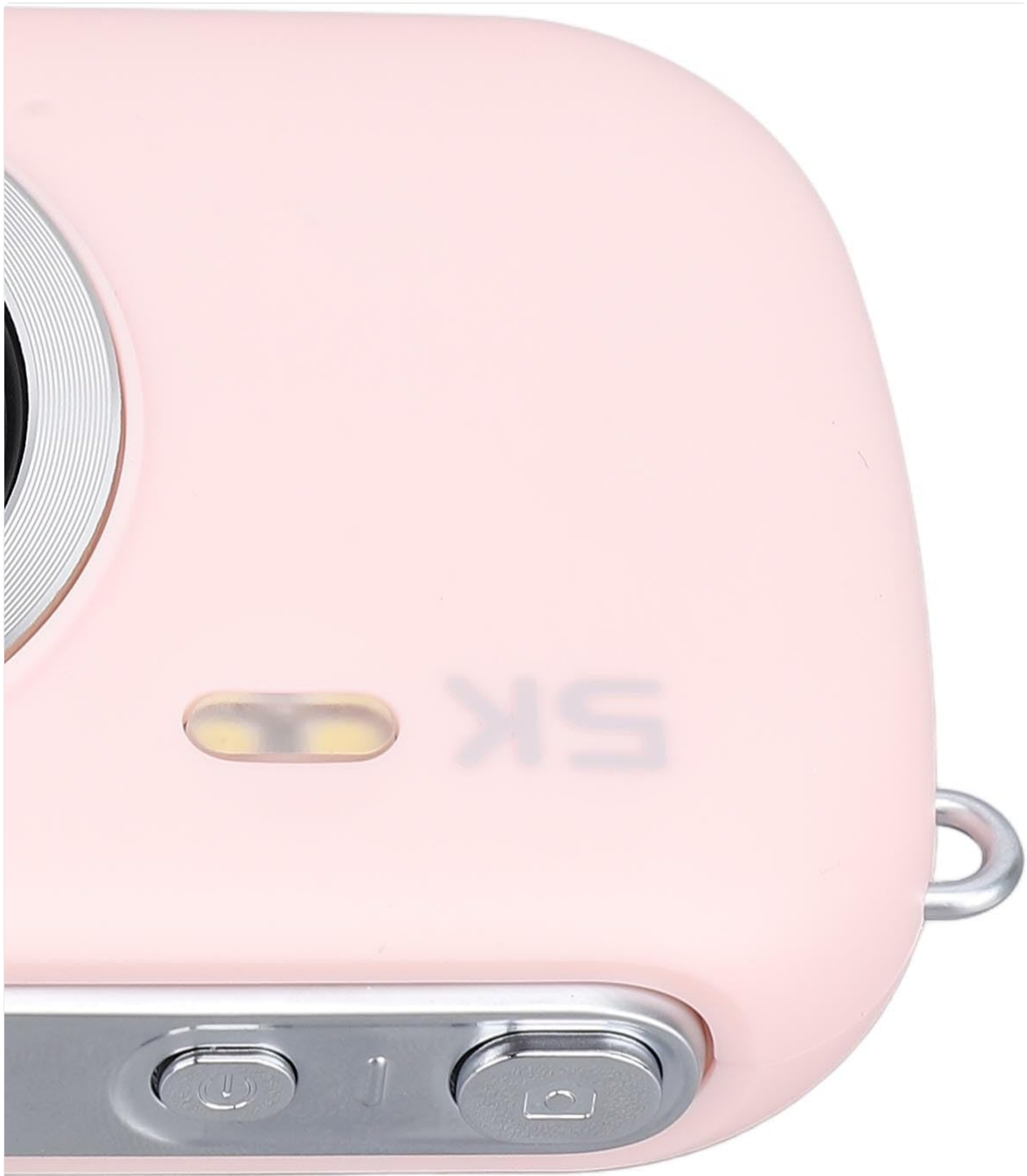
Figure 5.2: Location of the built-in flash.
