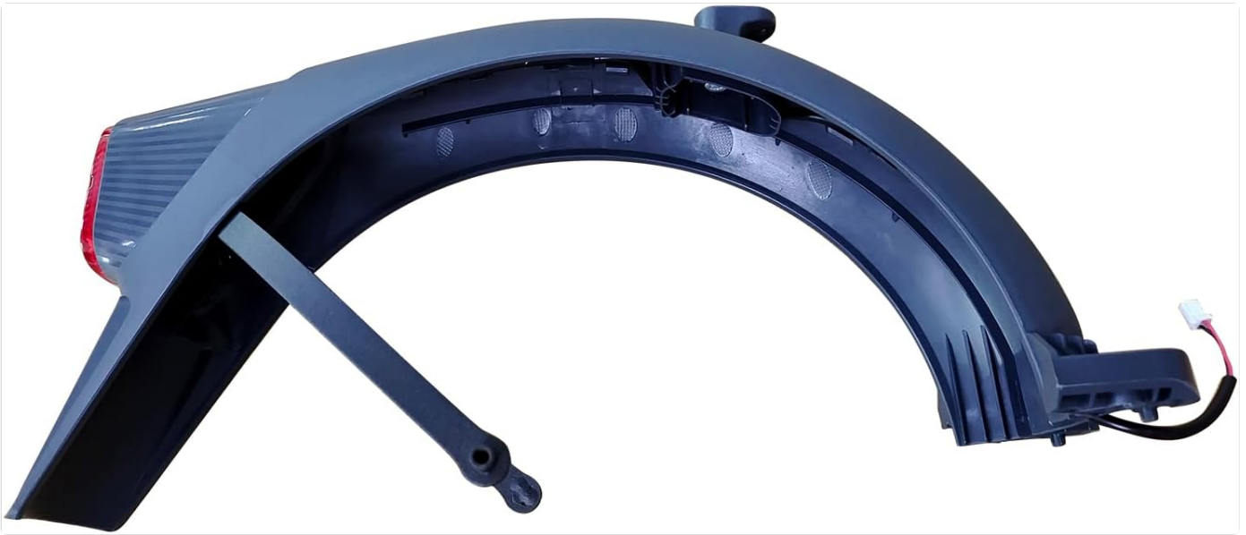
Figure 5: A detailed view of the integrated LED taillight on the XBERSTAR rear fender, highlighting its design for improved visibility and safety.
