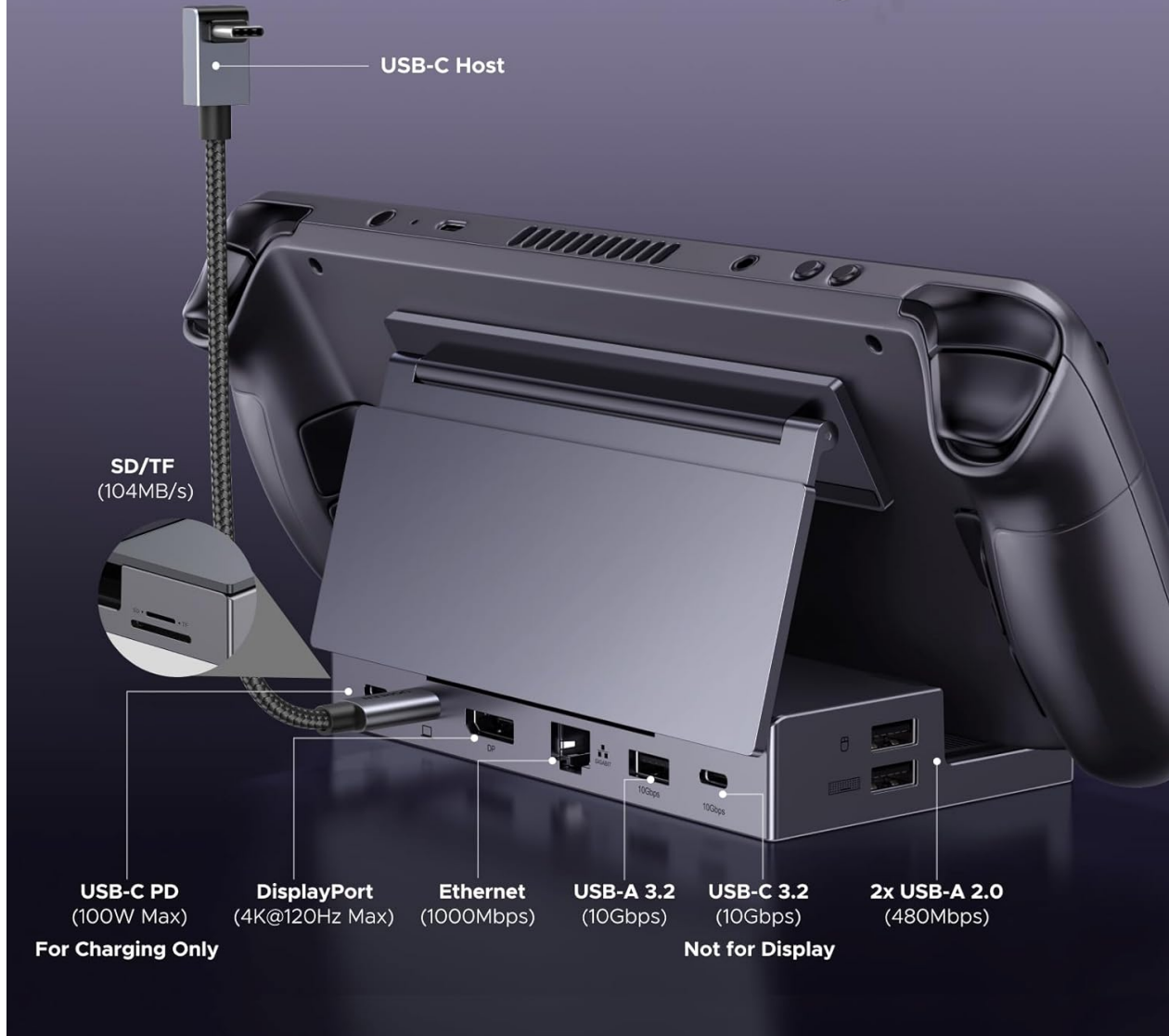
Figure 1: Overview of the UGREEN 9-in-1 Docking Station with labeled ports.
