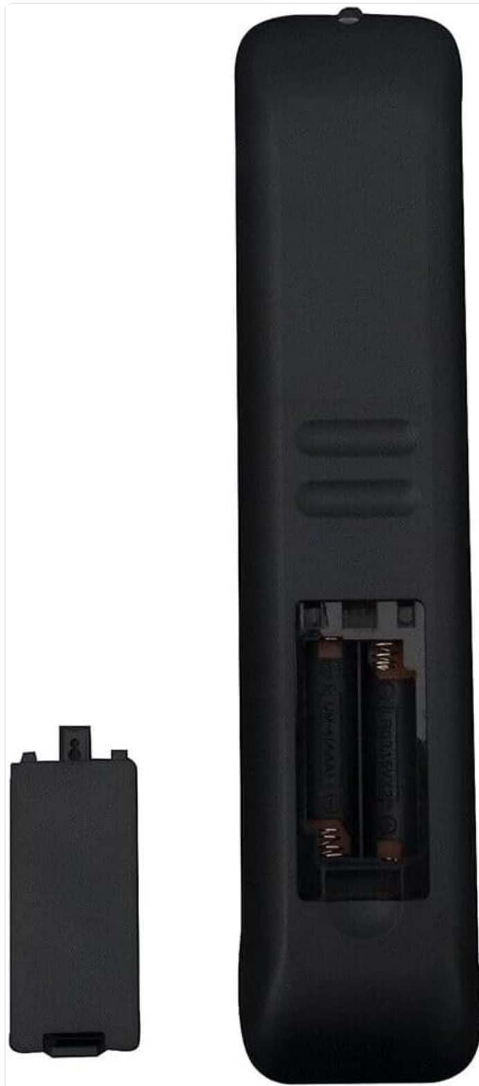
Image: Back of the remote control with the battery compartment open, illustrating correct battery placement.
