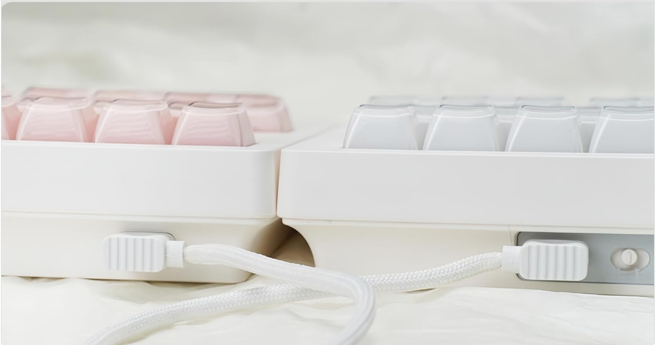
Image: Close-up of the split connection socket and the tri-mode connection switch on the ZMX GMK70 keyboard.
