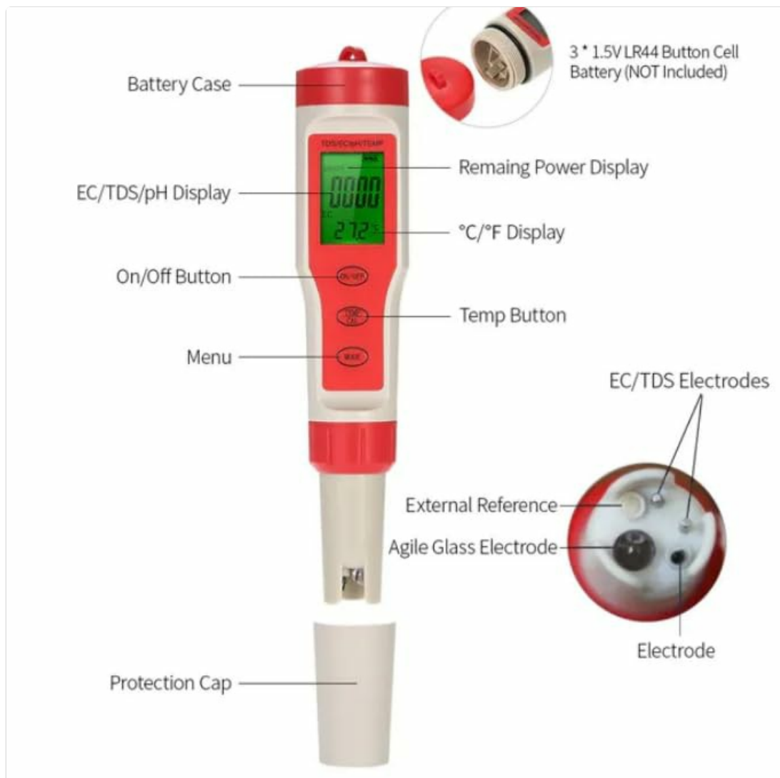
Detailed component diagram of the EZ9908 meter with battery information.
