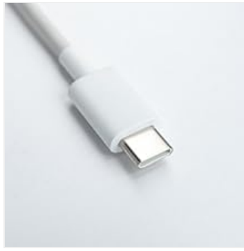
Figure 4.1: Type-C charging port.
