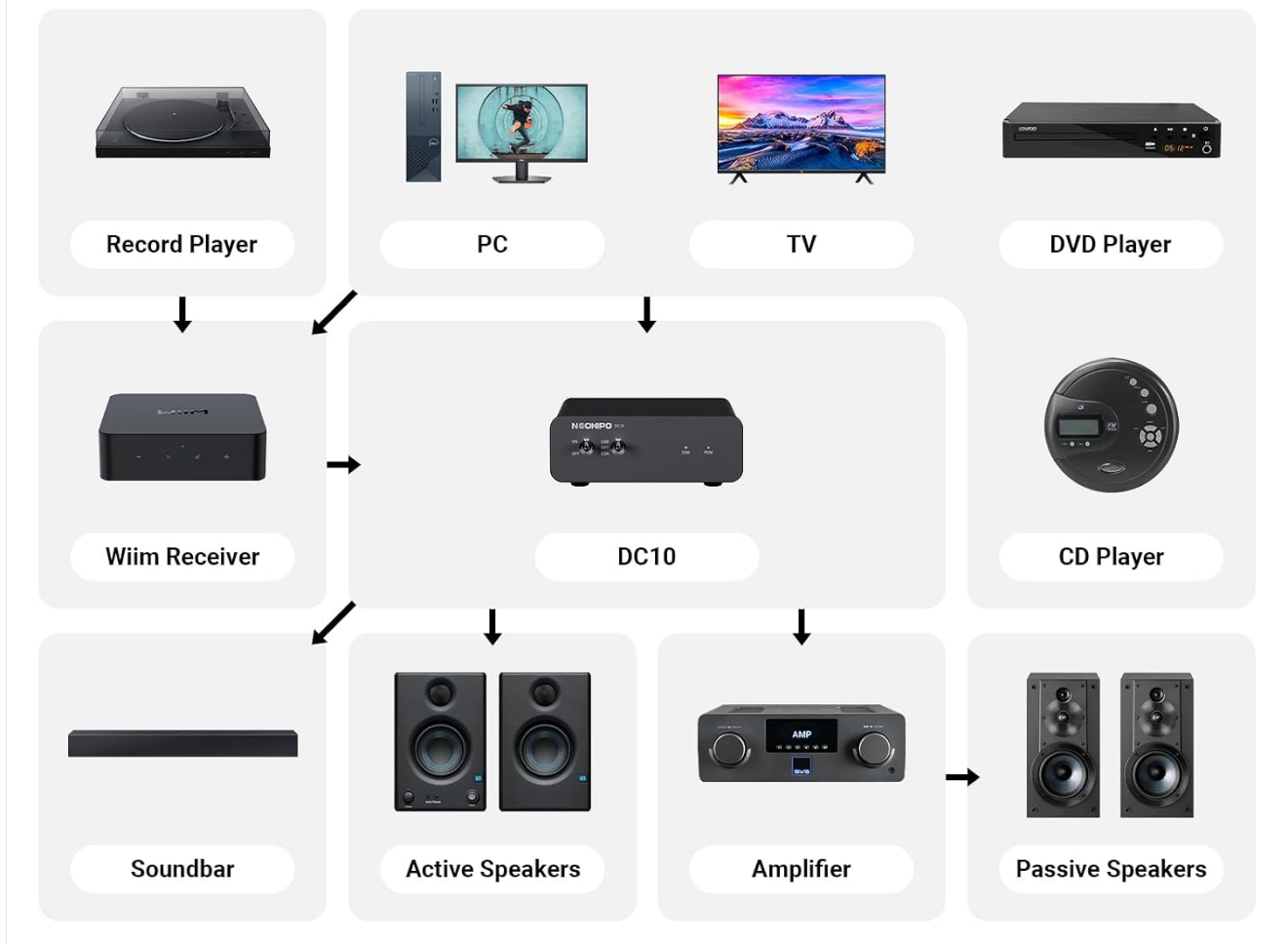
Figure 5: Connection diagram showing the versatility of the DC10 DAC with various audio sources and outputs.
