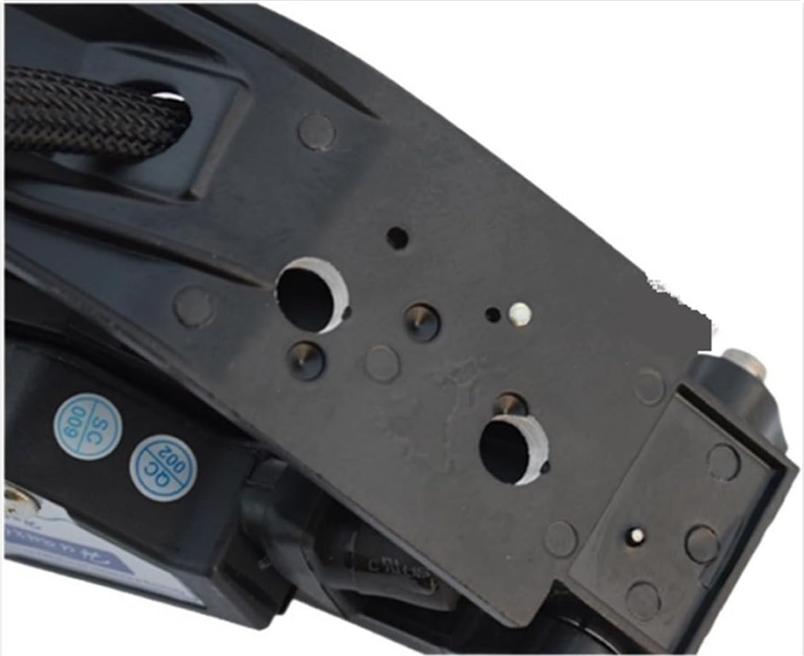
Figure 2: Underside view of the pedal, highlighting the mounting holes for secure attachment to the vehicle floor or frame.
